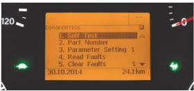
Advanced diagnostics system throws up fault indicators to the driver in the form of visual signals, messages and alarms to check for probable causes and take corrective action.
